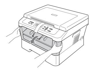
C Remove the Silica Pack from the inside of the machine.
