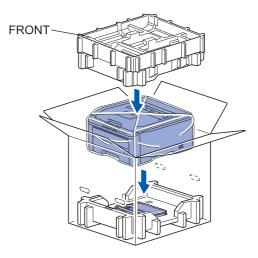
Put the power cord, drum unit and toner cartridge assemblies into the Styrofoam piece as shown in the illustration.
