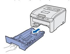
While pressing the green paper-guide release lever 1, slide the paper guides to fit the paper size you are loading in the tray. Make sure that the guides are firmly in the slots.
