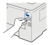
When this screen appears, turn on the printer's power switch.
