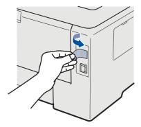
Connect the USB cable to the USB connector marked with a symbol, and then connect the cable to your Macintosh.
