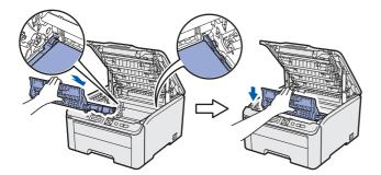
Reinstall the original packing material into the printer.
