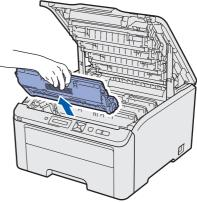
Attach the protective cover to each of the drum unit and toner cartridge assemblies.
