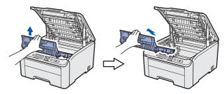
Remove the waste toner box from the printer, and then put it in a plastic bag and seal the bag completely.
