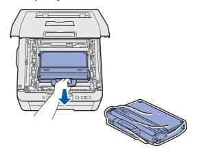
e Reinstall the belt unit back in the printer.
