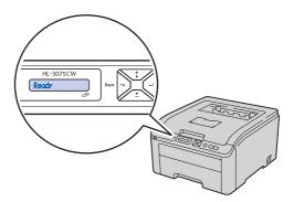
Press **Go**. The printer prints a test page. Check that the test page has printed correctly.
