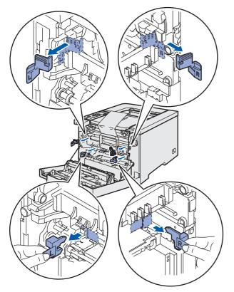
Hold the green handle of the drum unit. Lift the drum unit up and then pull it out until it stops.
