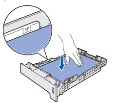
5 Put the paper tray firmly back into the printer. Make sure that it is completely inserted into the printer.
