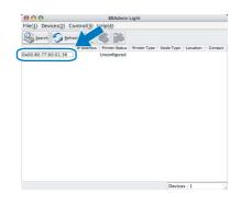
5 Choose Static for the Boot Method. Enter the IP Address, Subnet Mask and Gateway, and then click OK.
