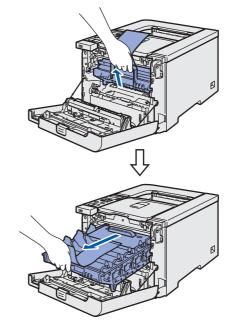
Remove the orange packing material as shown in the illustration below.
