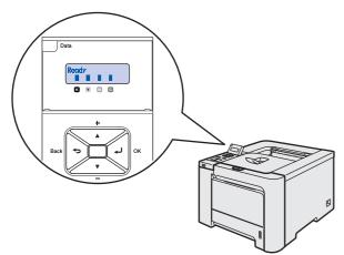
7 Press Go. The printer prints a test page. Check that the test page has printed correctly.
