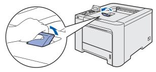
3 Make sure that the printer power switch is off. Remove the label covering the AC power inlet.
