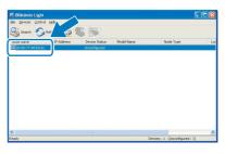
Choose **Static** for the **Boot Method**. Enter the **IP Address**, **Subnet Mask** and **Gateway**, and then click **OK**.
