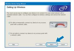
For configuration, you must temporarily connect your Brother wireless device (your printer) directly to a free port on your access point, hub or router using a network cable. When the following screen appears, insert the network cable to the access point and then to the printer. Click **Next**.
