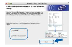
Click Finish. Wireless setup failed as it was unable to associate with a wireless network. This is probably due to incorrect security settings. Reset the print server back to its factory default settings (see page 43). Confirm the security settings that you wrote down on page 31 your wireless network and try starting from d on page 34 again.
