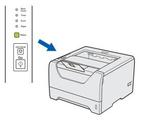
Press **Go**. The printer prints a test page. Check that the test page has printed correctly.
