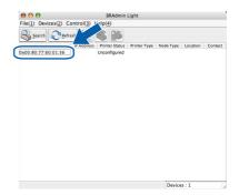
Choose **STATIC** for the **Boot Method**. Enter the **IP Address**, **Subnet Mask** and **Gateway**, and then click **OK**.
