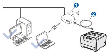
If there is an Ethernet Hub or Router in the same network as the wireless access point 1, you can temporarily connect the Hub or Router to the printer using an Ethernet cable 2. This is an easy way to configure the printer. You can then remotely configure the printer from a computer on the network.
