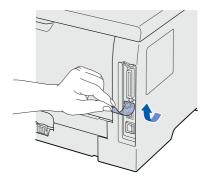
Press the wireless setup button located at the back of the printer for less than 2 seconds as shown in the illustration below. This will put the printer in one-push wireless setting mode. This feature will automatically detect which mode your access point uses for one-push configuration (SecureEasySetup™, Wi-Fi Protected Setup or AOSS™).
