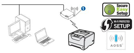
If your wireless access point ① supports either SecureEasySetup™, Wi-Fi Protected Setup (PBC ¹) or AOSS™, you can configure the printer without knowing your wireless network settings. The access point /router and your printer can automatically negotiate using the SecureEasySetup™, Wi-Fi Protected Setup or AOSS™ procedure.
