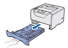
While pressing the blue paper-guide release lever 1, slide the paper guides to fit the paper size you are loading in the tray. Make sure that the guides are firmly in the slots.
