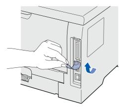
Connect the USB cable to the USB connector marked with a symbol, and then connect the cable to your Macintosh.
