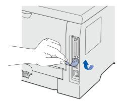
i When this screen appears, make sure the printer power switch is on. Connect the USB cable to the USB connector marked with a symbol, and then connect the cable to the computer. Click Next.
