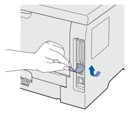
b Connect the USB cable to the USB connector marked with a - symbol, and then connect the cable to your Macintosh.
