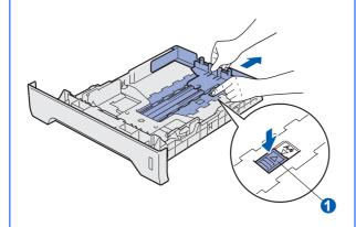
Fan the stack of paper well to avoid paper jams and misfeeds.
