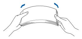
Put paper in the tray, and make sure that the paper is below the maximum paper mark 1. The side to be printed on must be face down.
