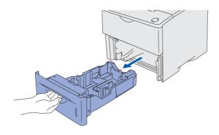
While pressing the paper guide release lever, slide the adjusters to fit the paper size. Check that the guides are firmly in the slots.
