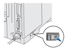
4 Connect the parallel interface cable to your PC, and then connect it to your printer.
