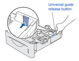
To avoid paper jams and misfeeds, fill the paper tray with small stacks of paper that you have fanned well.
