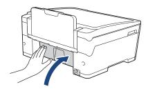
9. If your LCD error message was [Jam Front/MP Tray] or [Repeat Jam Front/MP Tray], make sure you look carefully inside the MP tray for jammed paper. Push the release lever (1) towards the back of the machine, and then slowly pull the jammed paper out of the MP tray.
