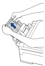
2. Gently press and slide the MP tray paper guides to match the width of the paper you are using.
