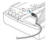
3. Carefully route the USB cable throught the trench and out the back of the machine as shown below.
