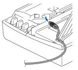
3. Carefully route the USB cable throught the trench and out the back of the machine as shown below.
