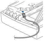
3. Carefully route the network cable through the trench and out the back of the machine as shown below.
