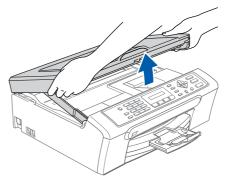
11 Insert the USB cable into the USB socket marked with a symbol. You will find the USB socket inside the machine as shown below.
