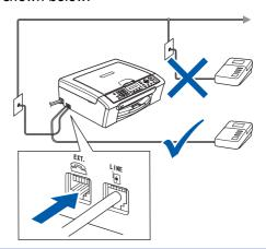
Set the receive mode to 'External TAD' if you have an external answering machine. For details, see Connecting an external TAD (telephone answering device) in Chapter 7 of the User's Guide.
