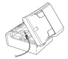
Carefully route the USB cable through the trench and out the back of the machine as shown below and connect the cable to your Macintosh<sup>®</sup>.
