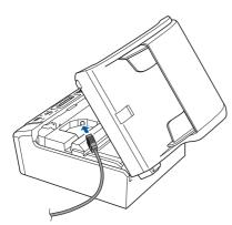
C Carefully route the USB cable through the trench and out the back of the machine as shown below and connect the cable to your computer.
