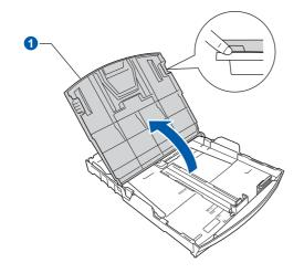
C With both hands, gently press and slide the paper side guides (1) and then the paper length guide (2) to fit the paper size.
