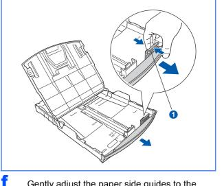
Gently adjust the paper side guides to the paper with both hands. Make sure that the paper side guides touch the edges of the paper.
