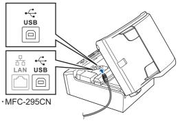
Carefully guide the USB cable through the trench as shown below, following the trench around and toward the back of the machine. Then connect the cable to your Macintosh.
