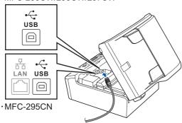
Carefully guide the USB cable through the trench as shown below, following the trench around and toward the back of the machine. Then connect the cable to your computer.
