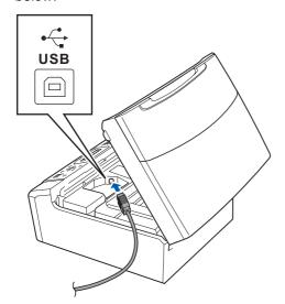
Carefully route the USB cable through the trench and out the back of the machine as shown below and connect the cable to your computer.
