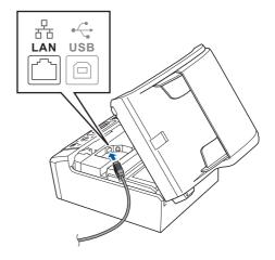
Carefully route the network cable through the trench and out the back of the machine. Then, connect the cable to your network.
