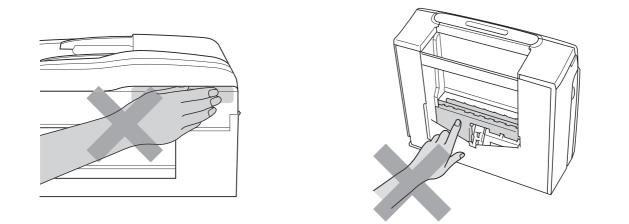
When moving the machine you must lift it from the base, by placing a hand at each side of the unit as shown in the illustration. DO NOT carry the machine by holding the scanner cover or the Jam Clear Cover.
