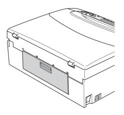
6 Lift the scanner cover (1) from the front side of the machine until it locks securely in the open position. Make sure that jammed paper is not left inside the machine.
