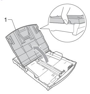
With both hands, gently press and slide the paper side guides (1) and then the paper length guide (2) to fit the paper size. Make sure that the triangular marks (3) on the paper side guides (1) and paper length guide (2) line up with the marks for the paper size you are using.
