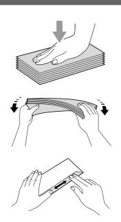
2 Put envelopes or postcards into the paper tray with the address side down and the leading edge in first as shown in the illustration. With both hands, gently press and slide the paper side guides (1) and paper length guide (2) to fit the size of the envelopes or postcards.
