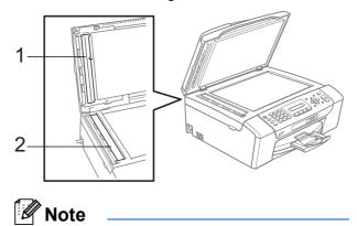
In addition to cleaning the scanner glass and glass strip with a non-flammable glass cleaner, run your finger tip over the glass to see if you can feel anything on it. If you feel dirt or debris, clean the glass again concentrating on that area. You may need to repeat the cleaning process three or four times. To test, make a copy after each cleaning attempt.
