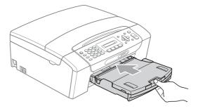
9 While holding the paper tray in place, pull out the paper support (①) until it clicks, and then unfold the paper support flap (②).
