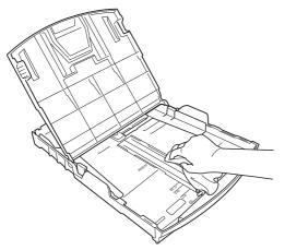
5 Close the output paper tray cover and put the paper tray firmly back in the machine.
