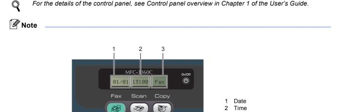
When the machine is idle (not being used) it will return to the default display shown above. The default display shows the date, time, and the current receive mode.
