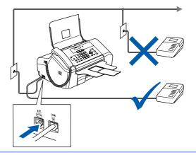
Set the receive mode to 'External TAD' if you have an external answering machine. For details, see Connecting an external TAD (telephone answering device) in Chapter 7 of the User's Guide.
