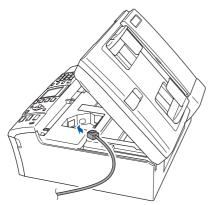
4 Carefully guide the network cable into the trench as shown below, following the trench around and toward the back of the machine. Then, connect the cable to your network.
