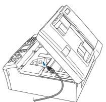
Carefully guide the USB cable into the trench as shown below, following the trench aound and toward the back of the machine. Then, connect the cable to your computer.
