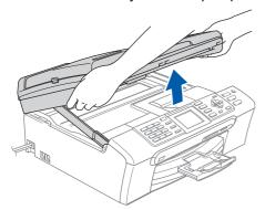
Insert the USB cable into the USB socket marked with a symbol. You will find the USB socket inside the machine on the right as shown below.
