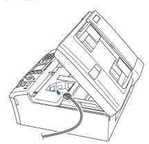
Carefully route the network cable through the trench and out the back of the machine.
