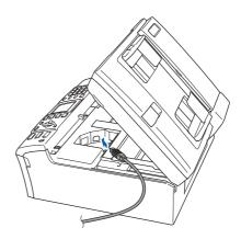
12 Carefully route the USB cable through the trench and out the back of the machine as shown below and connect the cable to your computer.
