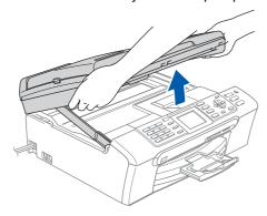
Insert the network cable into the LAN socket marked with a R symbol. You will find the LAN socket inside the machine on the left as shown below.
