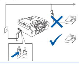
Set the receive mode to 'External TAD' if you have an external answering machine. For details, see Connecting an external TAD (telephone answering device) in Chapter 7 of the User's Guide.
