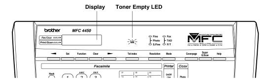
The Toner Empty LED will light and the display will show CHANGE TONER and TONER EMPTY alternately to indicate that the toner is empty. Once this indication appears, your MFC will not resume printing until you have installed a new toner cartridge.
