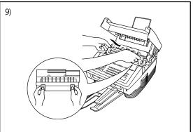
9) Reinstall the drumunit into the MFC and close the top cover. Then, turn on the power switch or plug in the power cord.
