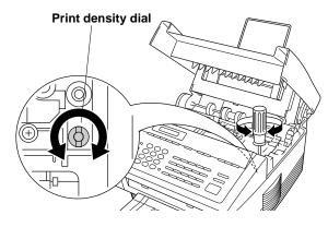
Use a straight blade screwdriver to turn the print density dial clockwise for darker print and counterclockwise for lighter print. The dial has been set to the middle position.
