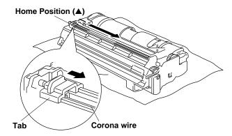
3 Return the tab to the home position (▲ mark position) before reinstalling the drum unit.
