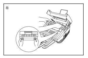
8) Holding the new drum unit by its handles, install it. Close the top over.
