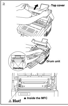
2) Open the top cover. To remove the drum unit, hold each side of the drum by its handles and gently lift the drum forward toward you.
