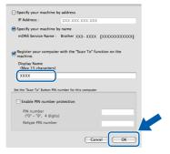
The name you enter will appear on the machine's LCD when you press the **Scan** key and choose a scan option. (For more information, see Network Scanning in the Software User's Guide on the CD-ROM.)
