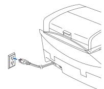
2 Connect the telephone line cord. Connect one end of the telephone line cord to the jack on the machine marked **LINE** and the other end to a modular wall jack.
