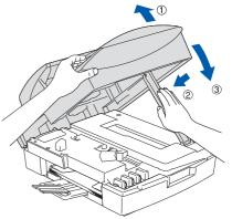
The machine will clean the ink tube system for use for the first time. This process will occur only once, the first time ink cartridges are installed. The cleaning process will last approximately four minutes. The LCD shows:
