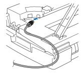
3. Carefully route the USB cable through the trench and out the back of the machine as shown below.
