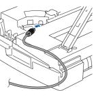
3. Carefully route the USB cable through the trench and out the back of the machine as shown below.
