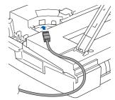
3. Carefully route the network cable through the trench and out the back of the machine as shown below.
