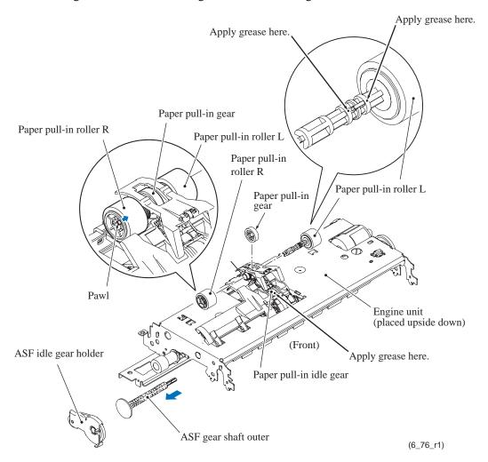
**Assembling Note:** Before mounting the paper pull-in roller L, apply the specified lubricant to the paper pull-in idle gear and paper pull-in roller L, referring to Section 6.2.
