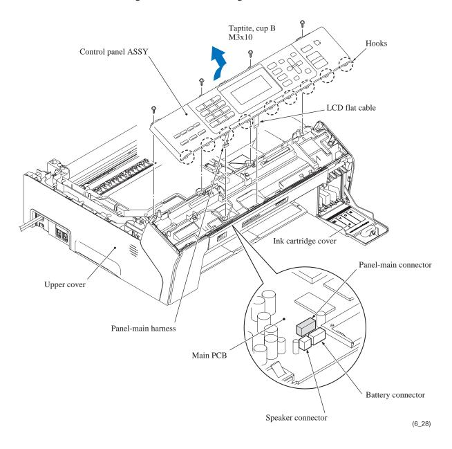
**Assembling Note:** After mounting the control panel ASSY, check that there is no gap between the front end of the control panel ASSY and that of the upper cover.
