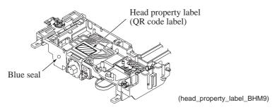
**Note:** Depending on whether the head/carriage unit has a round, blue seal on its left side, the purge type to be performed differs. Refer to Chapter 7, Section 7.2 [2].
