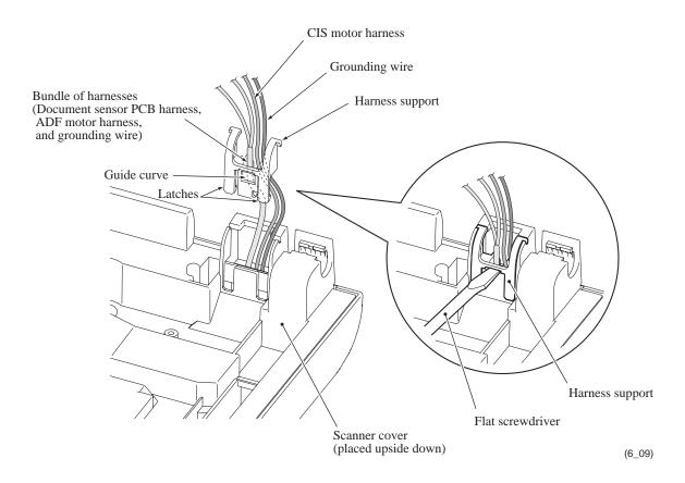
**Assembling Note:** Before fitting the harness support (shown above) into the scanner cover, route the document sensor PCB harnesses and the bundle of ADF motor harness and its grounding wire through the guide curve provided in the harness support. The CIS motor harness and the grounding wire should be placed at the rightmost position (viewed from the bottom) in the square opening in the scanner cover.
