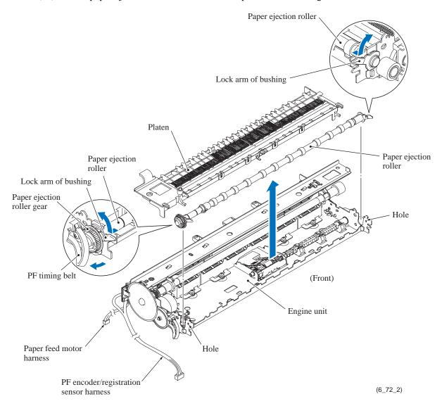
**Assembling Note:** When mounting the paper ejection roller, set its bushings into the engine chassis and turn their lock arms to fit the bosses on the lock arms into the holes provided in the engine chassis.
