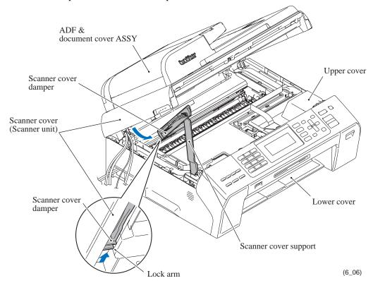
(8) Fully open the scanner cover and pull it to the rear and off the machine.
