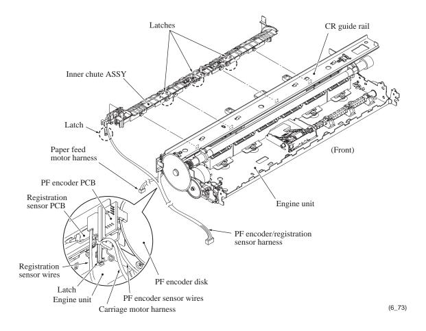
**Assembling Note:** When mounting the inner chute on the engine unit, first set the left two latches and then the rightmost one.
