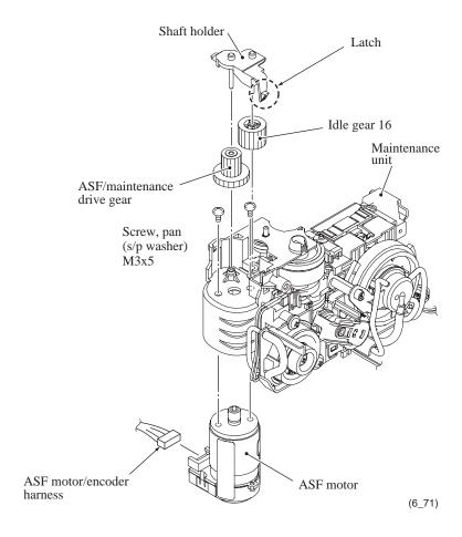
**Assembling Note:** When mounting the ASF motor on the maintenance unit, first fit the small hole of the ASF motor on the small boss inside the ASF motor holder, then secure the motor with the two screws.
