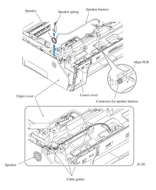
**Assembling Note:** After mounting the speaker and its spring into the pocket provided on the upper cover, route the speaker harness through the cable guides on the upper cover as shown on page 6-29.
