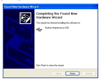
**NOTE:** In order to check whether the printer driver is successfully installed, click **Start** | **Settings** | **Printers** to select the Printers window. Then, check that the Brother Maintenance USB Printer icon is shown.
