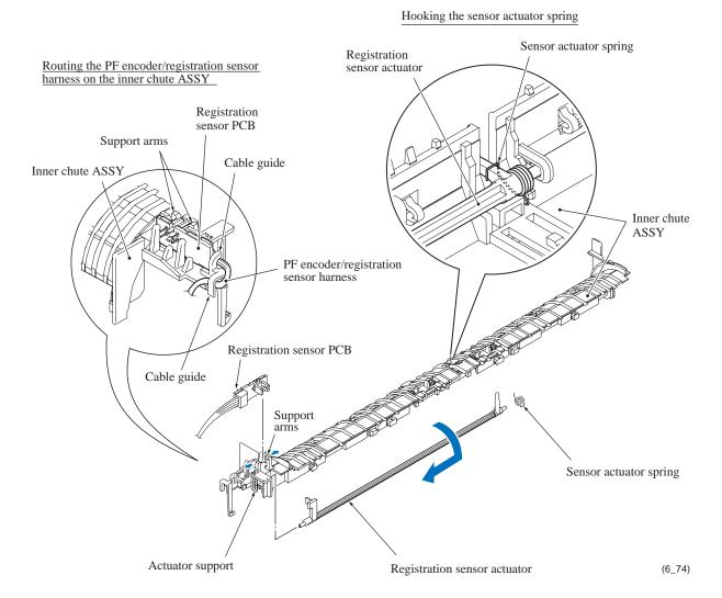
**Assembling Note:** Before mounting the inner chute on the engine unit, set the registration sensor actuator and its spring. Also set the registration sensor PCB and route the PF encoder/registration sensor harness as shown above.
