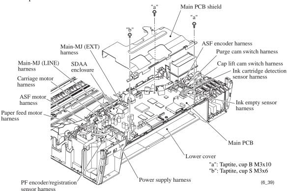
**Assembling Notes:** Before securing the main PCB shield, route the harnesses on the top of the lower cover as shown below. Make sure that the main-MJ (EXT) harness and main-MJ (LINE) harness are routed through the SDAA enclosure. (See the illustration given on page 6-40 for the routing of those harnesses on the left side of the lower cover.)
