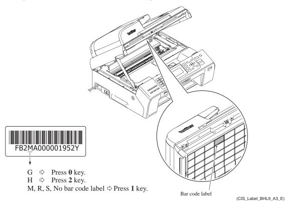
(2) Press the **5** and **9** keys in this order in the initial stage of the maintenance mode.
