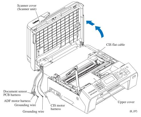
**Assembling Note:** If you replace the scanner cover, specify the CIS type into the EEPROM in the maintenance mode (Function code 59), referring to Chapter 9, Section 9.4.17. After that, acquire the white level data and set the CIS scanner area in the maintenance mode (Function code 55), referring to Chapter 9, Section 9.4.15.
