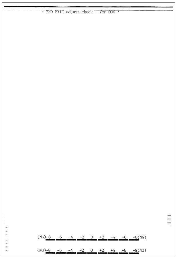
Paper Feeding Check Pattern for the Paper Ejection Roller
