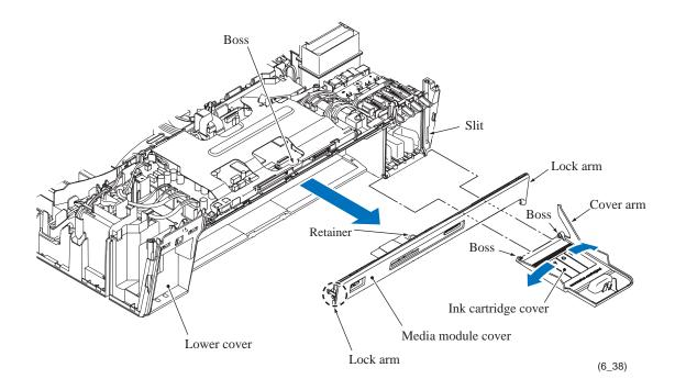
**Assembling Note:** When mounting the ink cartridge cover, first insert the cover arm into the slit provided in the right side of the lower cover and fit the right boss into the right hole in the lower cover. Then warp the center of the ink cartridge cover upward as shown above and fit the left boss into the left hole.
