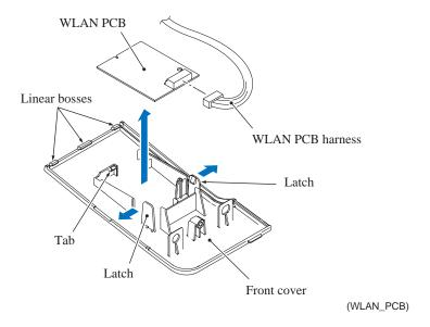
**Assembling Note\*:** When mounting the front cover and WLAN PCB onto the lower cover, route the WLAN PCB harness as shown on page 6-77.
