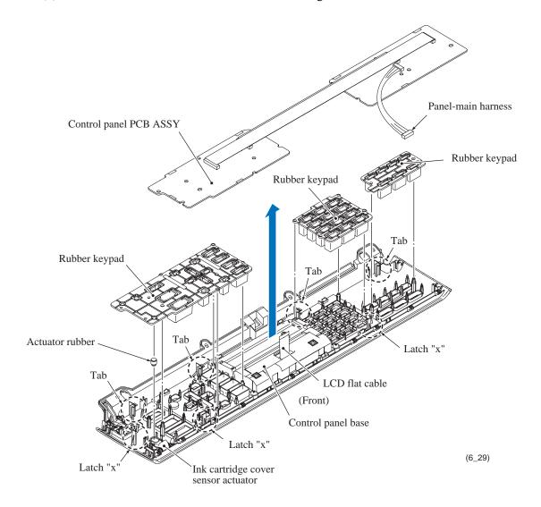
**Assembling Note:** When mounting the control panel PCB ASSY, first fit it below the four tabs (see the illustration above) on the control panel base and then secure it with three "x" latches.
