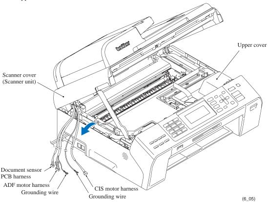
**Assembling Note:** Route the document sensor PCB harnesses, ADF motor harness, CIS motor harness, and grounding wires as shown below.
