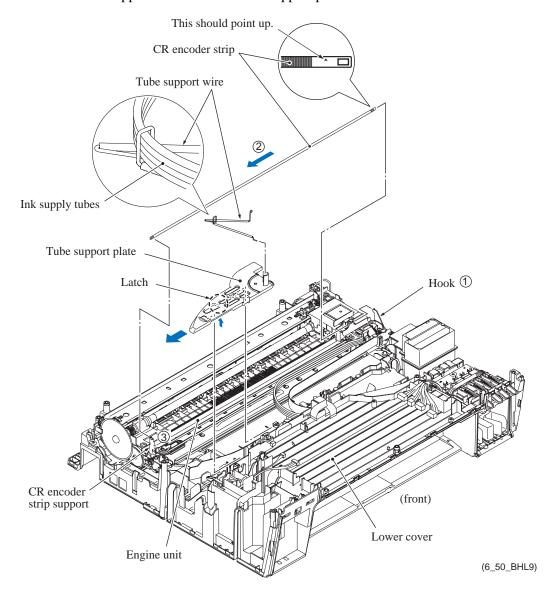
**Assembling Notes:** After mounting the head cover, set the CR encoder strip so that the ▲-marked end is to the right (carriage motor side) and the mark points upwards as shown above, using the following steps.
