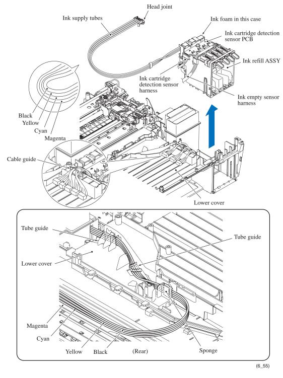
**Assembling Note:** After mounting the ink refill ASSY, route the ink supply tubes on the lower cover, aligning the four colors in the order as shown above.
