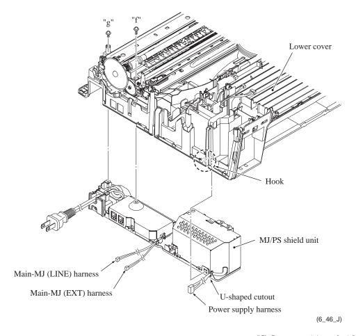
"f": Screw, pan (s/p washer) M3x8 "g": Taptite, cup S M3x6
