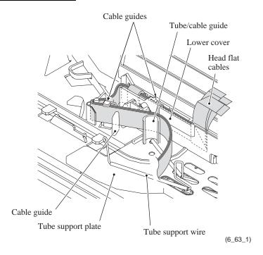
Routing I: Purge cam switch harness, cap lift cam switch harness, carriage motor harness, and ASF motor/encoder harness on the lower cover
