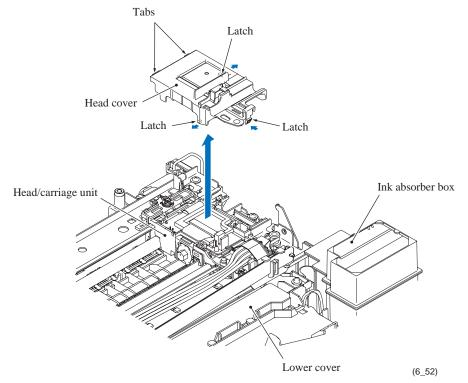
**Assembling Note:** When accessing the head/carriage unit placed on the engine unit, put the head/carriage unit in position "P" (on the right edge of the engine chassis) as shown above.
