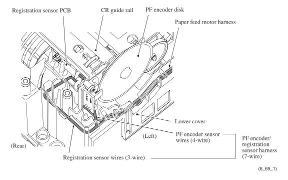
**Routing K:** ASF motor/encoder harness on the lower cover
