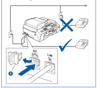
Set the receive mode to External TAD if you have an external answering machine. See Choose the correct Receive Mode on page 8. For additional details, see Connecting an external TAD (telephone answering device) in Chapter 7 of the User's Guide.
