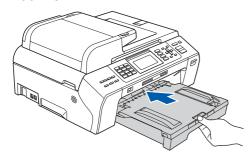
While holding the paper tray in place, pull out the paper support 1 until it clicks, and then unfold the paper support flap 2.
