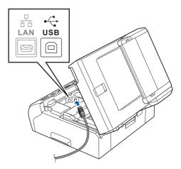
Carefully route the USB cable through the trench and out the back of the machine as shown below and connect the cable to your Macintosh.
