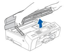
You will find the LAN socket marked with a symbol inside the machine on the left as shown below. Remove the protective cap and connect the network cable to the LAN socket.
