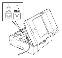
C Carefully route the USB cable through the trench and out the back of the machine as shown below and connect the cable to your computer.
