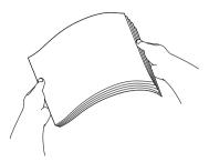
Gently insert the paper into the paper tray print side down and the leading edge (top of the paper) in first.
