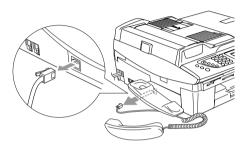
**2** Pull the knob to the left and hold it in position as you push the cradle to the back of the machine.
