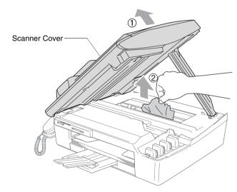
If the paper is jammed underneath the print head, disconnect the machine from the power source so you can move the print head to take out the paper.
