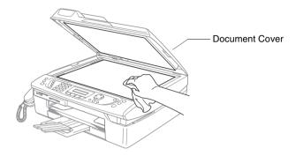
Clean the white bar and the glass strip under the film with isopropyl alcohol on a lint-free cloth.
