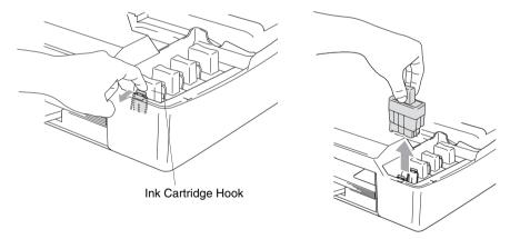
3 Open the new ink cartridge bag for the color shown on the LCD, and then take out the ink cartridge. 4 Remove the protective yellow caps.
