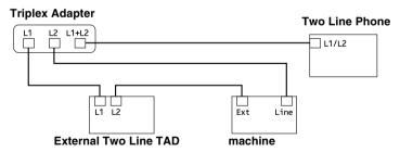
You can keep two-line telephones on other wall outlets as always. There are two ways to add a two-line telephone to the machine's wall outlet. You can plug the telephone line cord from the two-line telephone into the L1+L2 jack of the triplex adapter. Or, you can plug the two-line telephone into the TEL jack of the two-line TAD.
