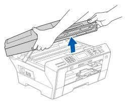
Connect the network cable to the LAN socket marked with a  $\mathbb{R}$  symbol. You will find the LAN socket inside the machine on the left as shown below.
