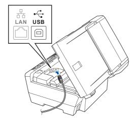
Carefully route the USB cable through the trench and out the back of the machine as shown below and connect the cable to your computer.
