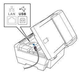
Carefully route the USB cable through the trench and out the back of the machine as shown below and connect the cable to your Macintosh<sup>®</sup>.
