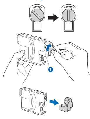
Take care to match the color of the lever 1 with the cartridge color 2, as shown in the diagram below.
