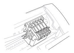
3 Open the ink cartridge cover by pinching the clip as shown in the illustration.
