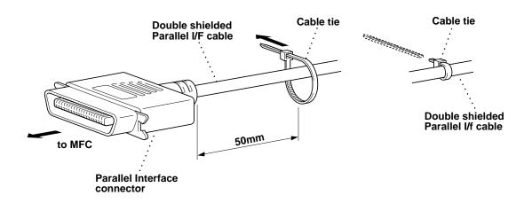
2 Attach the Filter core, pressing until you hear a click, between the Parallel Interface connector and the Cable tie.
