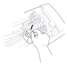
**7** Open the new ink cartridge bag for the colour on the display and remove the ink cartridge.
