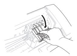
**10** After installing all ink cartridges, close the top cover until it clicks into place. Your MFC now prepares for a "head cleaning" and goes online. The MFC will ask you if you changed each colour ink cartridge.
