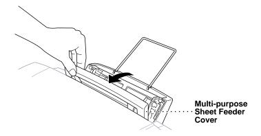
**B** Fan the paper well. Load the paper. Make sure the printing surface is towards you and the paper level is stacked below the paper guide line.
