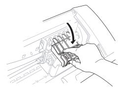
11 After installing the ink cartridges, close the top cover. Your MFC prepares for a "head cleaning" and goes online. The display screen prompts you to verify a new ink cartridge was inserted for each color you removed. Example: DID YOU CHANGE BLCK 1. YES 2. NO.
