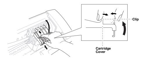
**6** Remove the ink cartridge by lifting it up and then out of the print head.
