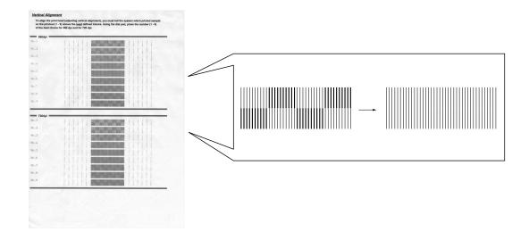
3 Select the best aligned print sample (1 to 9) for 360 and 720 dpi by using the Up/Down scroll control.
