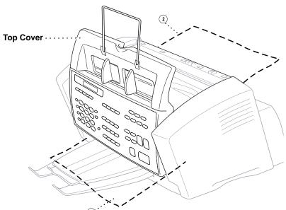
**2** Lift the top cover and make sure where the paper is jammed.
