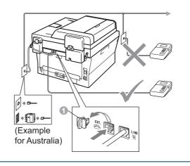
Set the receive mode to External TAD if you have an external answering machine. See Choose a Receive Mode on page 9. For additional details, see Connecting an external TAD in the Basic User's Guide.
