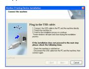
f Connect the USB cable to the USB connector marked with the symbol on your machine and then connect the cable to your computer.
