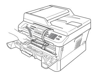
Pull the paper strip to remove the protective material as shown in the illustration.
