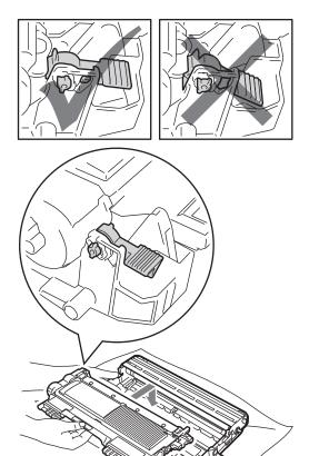
8 Put the drum unit and toner cartridge assembly back in the machine.
