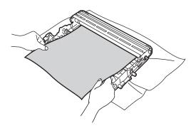
5 Turn the drum unit gear by hand while looking at the surface of the OPC drum (1).
