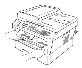
Using both hands, put one piece of A4 or Letter size paper in the manual feed slot until the top edge of the paper touches the paper feed roller. When you feel the machine pull in the paper, let go. The machine will start the Drum Cleaning process.
