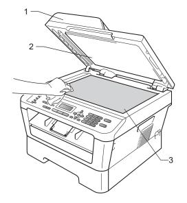
In the ADF unit, clean the white bar (1) and the glass strip (2) underneath it with a soft lint-free cloth moistened with water.
