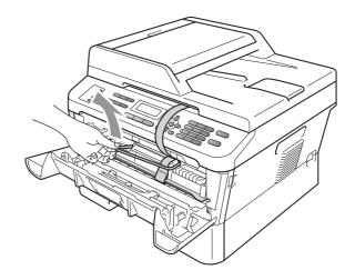
Pull the paper strip to remove the protective material as shown in the illustration.
