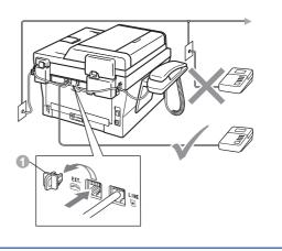
Set the receive mode to  ${\tt External}\ {\tt TAD}\ if$ you have an external answering machine. See Choose a Receive Mode on page 7. For additional details, see Connecting an external TAD in the Basic User's Guide.
