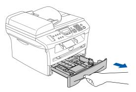
2 While pressing the paper guide release lever, slide the adjusters to fit the paper size. Check that the guides are firmly in the slots.
