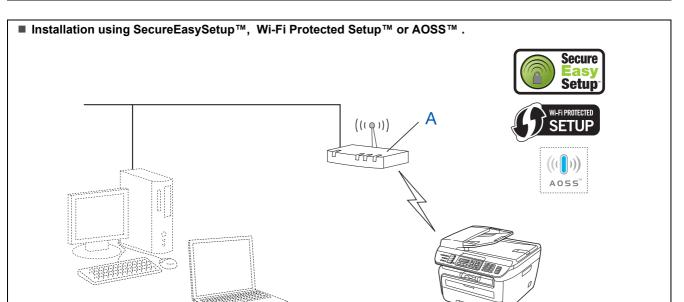
If your wireless access point (A) supports SecureEasySetup $^{TM}$ , Wi-Fi Protected Setup $^{TM}$  or AOSS $^{TM}$ , you do not need to use a computer to configure the machine. The access point (router) and your machine can automatically negotiate using the SecureEasySetup $^{TM}$  procedure. For instructions, go to page 25.
