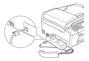
Pull the tab (1) back and hold it in position as you push the cradle (2) to the back of the machine.
