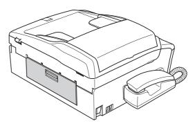
6 Lift the scanner cover (1) from the front side of the machine until it locks securely into the open position. Make sure that there is no jammed paper left inside the machine.
