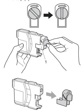
5 Each color has its own correct position. Insert the ink cartridge in the direction of the arrow on the label.
