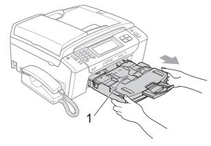
2 Pull out the jammed paper (1) and press **Stop/Exit**.
