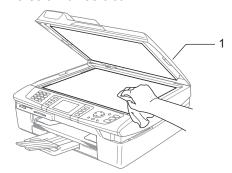
2 In the ADF unit, clean the white bar (1) and the glass strip (2) under it with isopropyl alcohol on a lint-free cloth.
