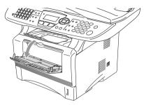
Using both hands put paper in the manual feed tray until the front edge of the paper touches the paper feed roller. Hold the paper in this position until the MFC automatically feeds the paper in for a short distance, and then let go of the paper.
