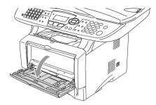
2 Pull out and unfold the MP tray support flap.
