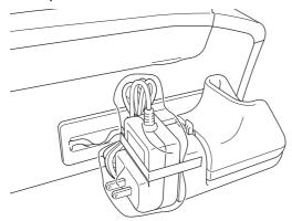
Route the AC power cord through the guide on the side of the machine. Then, plug the adapter into an AC power outlet.
