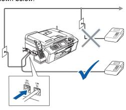
Set the receive mode to 'Manual' if you have an external answering machine. For details, see Connecting an external TAD (telephone answering device) in Chapter 7 of the User's Guide.
