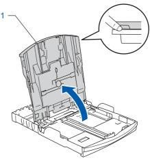
Press and slide the paper side guides (1) and paper length guide (2) to fit the paper size.
