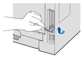
Connect the USB cable to the USB connector on the machine marked with the especial symbol. Then connect the cable to your computer.
