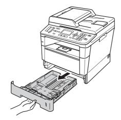
While pressing the green paper-guide release lever ①, slide the paper guides to fit the paper size you are loading in the tray. Make sure that the guides are firmly in the slots.
