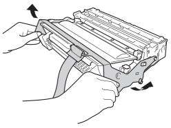
Hold the drum unit and toner cartridge assembly level with both hands and gently shake it from side to side several times to distribute the toner evenly inside the cartridge.
