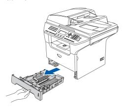
While pressing the paper guide release lever (1), slide the adjusters to fit the paper size. Check that the guides are firmly in the slots.
