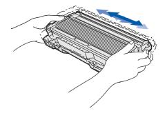
4 Put the drum unit assembly into the machine until it clicks into place.
