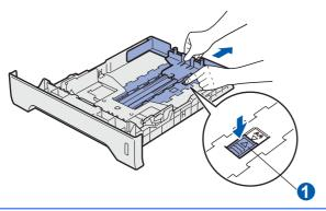
C Fan the stack of paper well to avoid paper jams and misfeeds.
