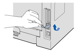
Connect the USB cable to the USB connector on the machine marked with the 😪 symbol. Then connect the cable to your computer.
