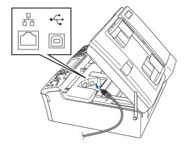
Carefully route the USB cable through the trench and out the back of the machine as shown below and connect the cable to your Macintosh®.
