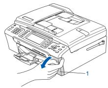
Pull all the lock release levers down and remove the yellow protective part (1).
