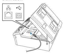
Carefully route the network cable through the trench and out the back of the machine. Then, connect the cable to your network.
