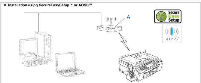
If your wireless access point (A) supports SecureEasySetup™ or AOSS™, you do not need to use a computer to configure the machine. The access point (router) and your machine can automatically negotiate using the SecureEasySetup™ or AOSS™ procedure.
