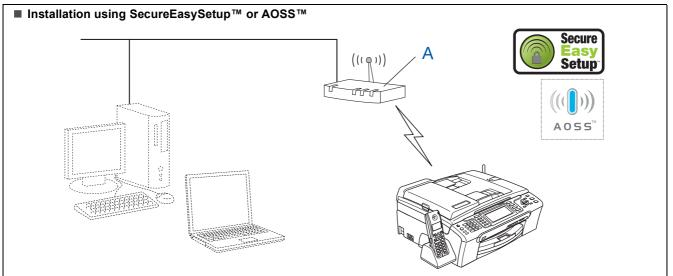
If your wireless access point (A) supports SecureEasySetup $^{\text{TM}}$  or AOSS $^{\text{TM}}$ , you do not need to use a computer to configure the machine. The access point (router) and your machine can automatically negotiate using the SecureEasySetup $^{\text{TM}}$  or AOSS $^{\text{TM}}$  procedure.
