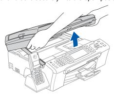
Insert the network cable into the LAN socket marked with a **R** symbol. You will find the LAN socket inside the machine on the left as shown below.
