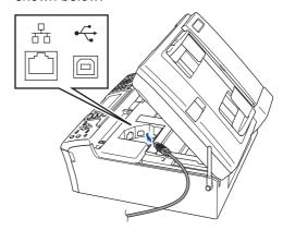
12 Carefully route the USB cable through the trench and out the back of the machine as shown below and connect the cable to your computer.
