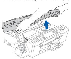
Insert the network cable into the LAN socket marked with a  $\mathbb{R}$  symbol. You will find the LAN socket inside the machine on the left as shown below.
