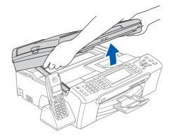
Insert the USB cable into the USB socket marked with a 😝 symbol. You will find the USB socket inside the machine on the right as shown below.
