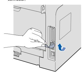
Connect the USB cable to the USB connector on the machine marked with the symbol. Then connect the cable to your computer.
