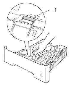
5 Wipe the two pick-up rollers (1) inside of the machine to remove dust.
