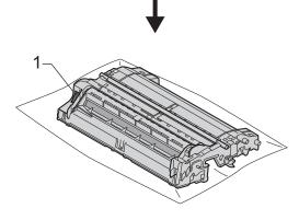
12 Use the numbered markers next to the drum roller to find the mark. For example, a dot in column 2 on the check sheet would mean that there is a mark in the "2" region of the drum.
