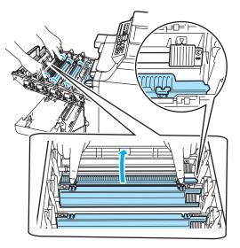
4 Repeat step 1 through step 3 to clean each of the remaining three corona wires.
