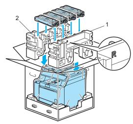
16 Put the carton tray (1) on the top. Match the front side of the machine to the Δ marks on the carton tray. Place the waste toner box in the right side of the carton tray.
