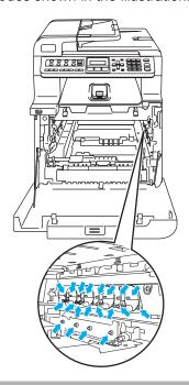
The jammed paper may be pulled out with the toner cartridge and drum unit assembly, or this may release the paper so you can pull it out of the paper tray opening.
