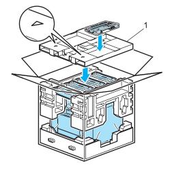
Put the four joints (1) into the holes of the carton using steps A and B as shown below.
