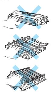
4 Hold the handle of the toner cartridge and pull it out of the drum unit. Repeat this for all the toner cartridges.
