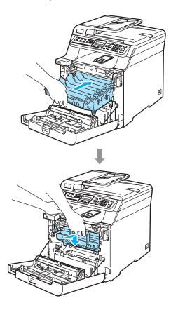
Insert the original orange packing material for the drum unit until as shown in the illustration, and then close the front cover.
