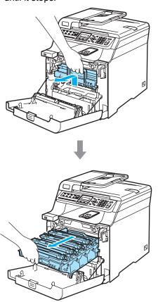
3 Release the gray lock lever (1) that is on the left side of the machine. Lift the front of the drum unit and pull the drum unit completely out of the machine using the green handles on the drum unit.
