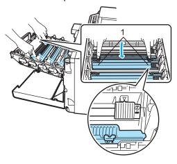
Clean the corona wire inside the drum unit by gently sliding the green tab from left to right and right to left several times.
