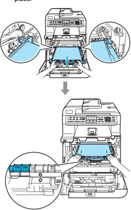
Insert the original orange packing material for locking the belt unit as shown in the illustration.
