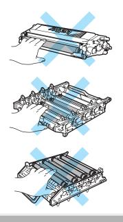
Turn the drum unit over by holding the green handles. Make sure that the drum unit gears (1) are on the left hand side.
