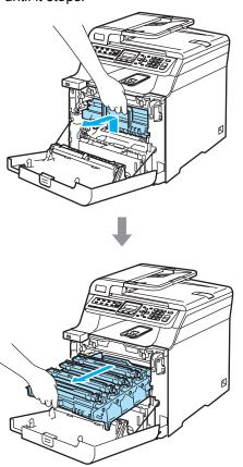
4 Release the gray lock lever (1) that is on the left side of the machine. Lift the front of the drum unit and pull the drum unit completely out of the machine using the green handles on the drum unit.
