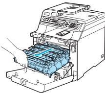
4 Hold the handle of the toner cartridge and pull it out of the drum unit. Repeat this for all the toner cartridges.
