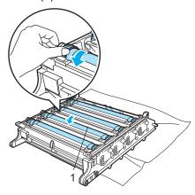
When you have found the mark on the drum that matches the print sample, wipe the surface of the drum gently with a dry cotton swab until the dust or paper powder on the surface comes off.
