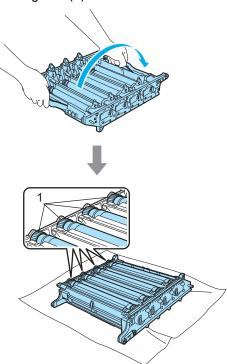
See the print sample to identify the color causing the problem. The color of the spots or toner stain is the color of the drum you should clean. For example, if the spots are cyan, you should clean the drum for cyan. Put the print sample in front of the drum, and the find the exact position of the poor print.
