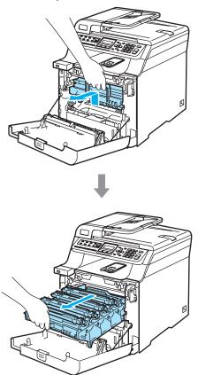
Release the gray lock lever (1) that is on the left side of the machine. Lift the front of the drum unit and pull the drum unit completely out of the machine using the green handles on the drum unit.
