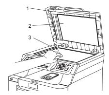
In the ADF unit, clean the white bar (1) and the scanner glass strip (2) underneath it with a soft lint-free cloth moistened with a non-flammable ammonia-free glass cleaner.
