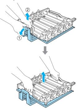
6 Hold the handle of the toner cartridge and slide the toner cartridge into the drum unit. Make sure that you match the toner cartridge color to the same color label on the drum unit, and make sure that you fold down the toner cartridge handle (A) once the toner cartridge is in place. Repeat this for all the toner cartridges.
