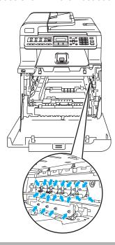
Hold the green parts of the belt unit with both hands and lift the belt unit up, then pull it out.
