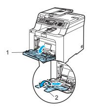
4 Put a blank sheet of A4 or Letter sized paper in the MP tray.
