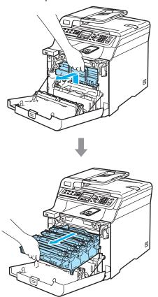
5 Release the gray lock lever (1) that is on the left side of the machine. Lift the front of the drum unit up and pull the drum unit completely out of the machine using the green handles on the drum unit.
