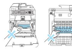
1 Press the front cover release button and then open the front cover.
