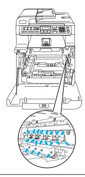
Hold the handles of drum unit when you carry it. DO NOT hold the sides of the drum unit.
