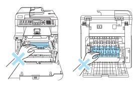
5 Using both hands, gently pull the jammed paper out of the fuser unit.
