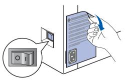
2 Connect the AC power cord to the machine.
