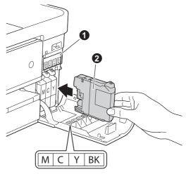
Gently push the back of the ink cartridge marked "PUSH" until the cartridge lever lifts. After all the ink cartridges are installed close the ink cartridge cover.
