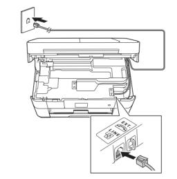
Connect the telephone line cord. Use the socket marked LINE and guide the cord out the back of the machine.
