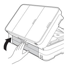
Lift the scanner cover (1) to release the lock. Gently push the scanner cover support down (2) and close the scanner cover (3) using both hands.
