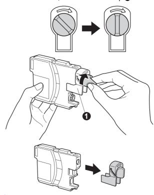
Take care to match the color of the lever with the cartridge color 2, as shown in the diagram below.
