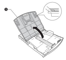
With both hands, gently press and slide the paper side guides • and then the paper length guide • to fit the paper size.
