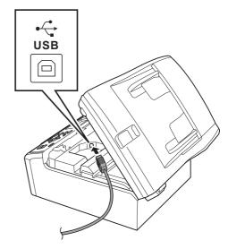
Carefully route the USB cable through the trench and out the back of the machine as shown below and connect the cable to your Macintosh.
