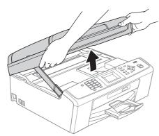
Connect the USB cable to the USB socket marked with a symbol. You will find the USB socket inside the machine as shown below.
