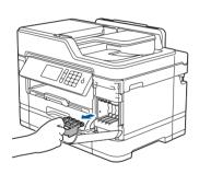
Open the ink cartridge cover, and then remove the orange protective part from the machine.
